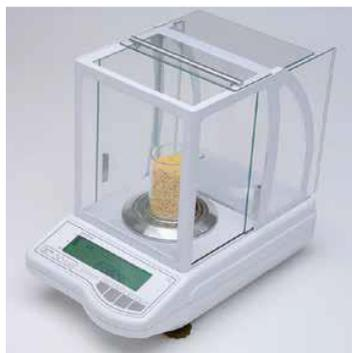
**Figura 4. Balanza Gibertini Crystal 200CAL**
